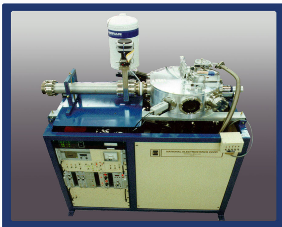
Model RC43 Analysis Endstation for PIXE, NRA and RBS with Channeling.
