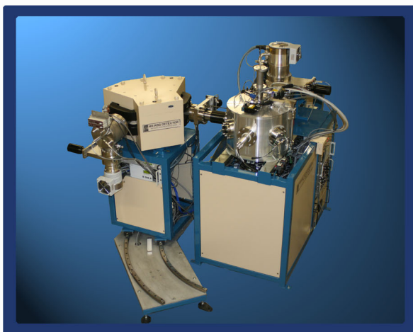
High Resolution RBS Detector attached to the model RC43 Analysis Endstation with angle variability of \pm 5^\circ at each 90^\circ and 135^\circ port.
