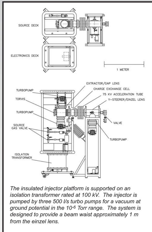
The insulated injector platform is supported on an isolation transformer rated at 100 kV. The injector is pumped by three 500 l/s turbo pumps for a vacuum at ground potential in the  $10^{-6}$  Torr range. The system is designed to provide a beam waist approximately 1 m from the einzel lens.
