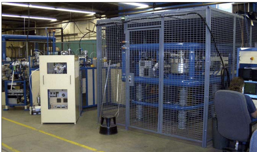
Figure 2 SSAMS system for the Radiocarbon Laboratory at the Geobiosphere Science Center, Lund, Sweden, during factory tests. The larger (blue) 300kV deck for the prototype tests is in the background to the left of the SSAMS.
