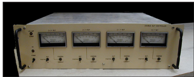
The local slit controller has switchable analog meters which display the slit position and current read.
