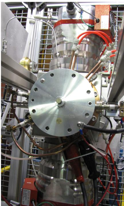
NEC's high current negative light ion injector is designed for use with tandem electrostatic accelerators. Dependent on version, the injector is capable of producing hydrogen (protons), deuterium, and helium ions.
