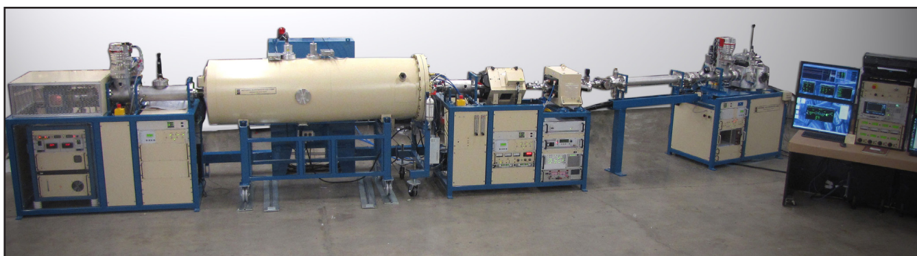
NEC Model 3SDH, which includes a RF charge exchange source (alphatross), 3SDH Pelletron, analysis beamline, and NEC RC43 analysis end station.
