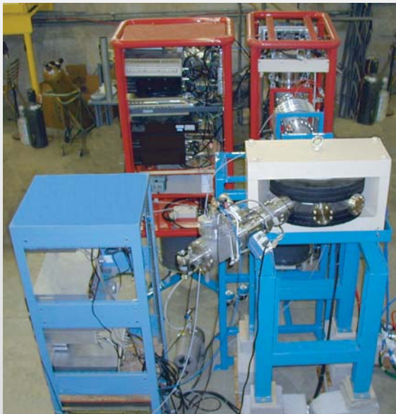
Experimental set up - The injector is in the background directly behind the +/-30° mass analyzer magnet. The negative ion beam current is measured in a suppressed, high power, tantalum Faraday cup in the foreground.
