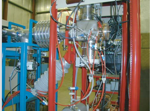
The TORVIS source is mounted to the far right followed by the extractor/gap lens assembly pumped by two 500 l/s turbo molecular pumps. The Rb cell immediately follows this assembly at the entrance to the 75 kV all metal/ceramic acceleration tube.
