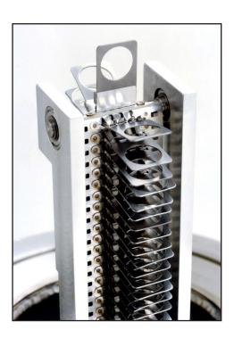
The NEC foil/target changer has been in manufacture for over two decades. Its unique design has found wide acceptance in accelerator laboratories throughout the world. At the present time, over 130 units have been shipped. It is ultra-high vacuum compatible with no moving seals. Units with as few as 48 positions and as many as 360 positions have been manufactured.
