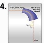
The positive ions are accelerated into the 90° mass/energy analysis magnet which separates the isotope beams for measurement.
