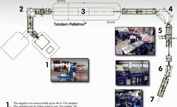
The negative ion source holds up to 40 or 134 samples. The samples can be either solid or gas. For carbon, the source produces a beam of carbon isotopes (\(^{12}C^{-},^{13}C^{-},^{14}C^{-}) and negatively charged molecules. This source is also suitable for studies with other radioisotopes.
