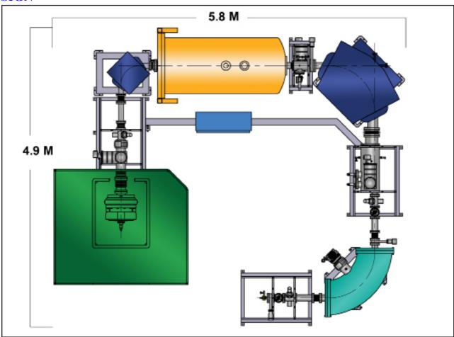
The NEC CAMS is designed for high precision measurement of carbon radioisotope ratios. This is a complete system with all necessary hardware and software for both on-line and off-line radiocarbon isotope ratio measurements.
