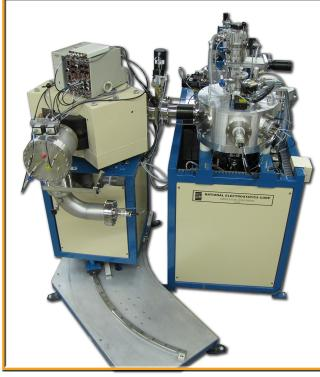
The HR-RBS detector system attaches to the NEC RC43 Analysis Endstation. The detector consists of an entrance aperture to define the scattering angle, a single focusing 90° magnet to resolve the energy of each scattered ion, and a position sensitive micro channel plate detection system to count the ions as a function of position. It can easily be positioned at the 90° or 45° port of the endstation. The bellows allows angle variability of ±5° at either port.
