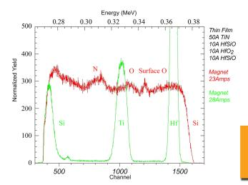
The spectra are modeled by the NEC RC43 software to provide elemental composition vs. depth profiles. ASCII spectra files can be imported into numerous data analysis packages.
