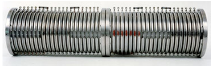
One million Volt assembly of high gradient acceleration tube sections designed for operation in 80 psig SF 6 insulating gas.
