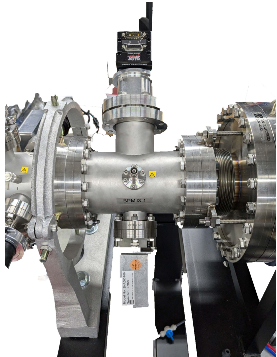
The original NEC low current beam profile monitor, Model BPM90-LC.
