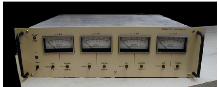
The local slit controller has switchable analog meters which display the slit position and current read.
