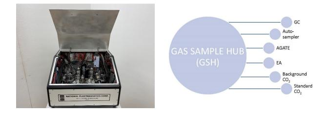
The design aim of the AGATE is to process between 40 and 100 samples in 24 hours, depending on the precision required. Other ampule commercial handing devices handle 8-10 samples and may experience problems with glass shards. The new AGATE automatically discards the broken ampules into a waste bin before processing the next sample. The current magazine capacity is 30 ampules, with higher-capacity magazines possible in future versions.
